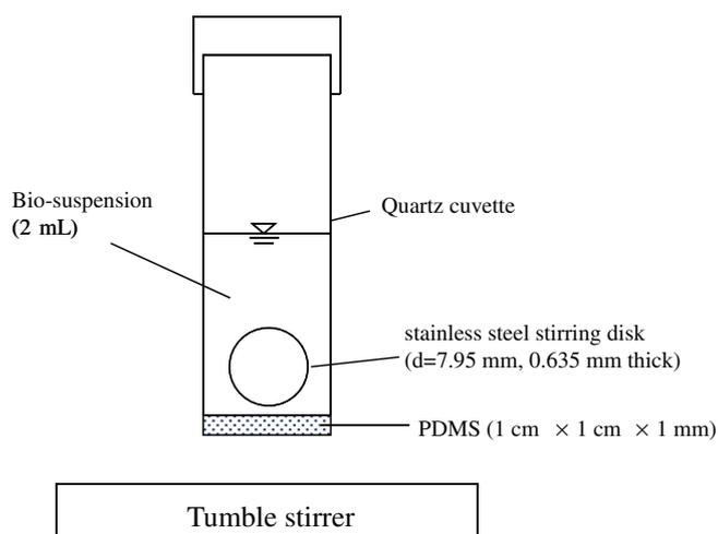
Fig. 1. Schematic diagram of the partition controlled delivery system used in this study.
